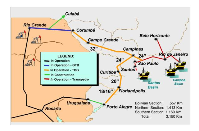
The gas pipeline has a diameter of 32 inches along the section from Rio Grande until Campinas (São Paulo state), where it forks into two sections of 24 inches each. The first fork ends at Guararema (São Paulo) where it links up with the existing gas pipeline system in Brazil's Southeast; the second fork flows south to Araucária in Paraná state. From Araucária until Porto Alegre (Rio Grande do Sul) the diameter of the pipeline becomes successively smaller until it reaches 16 inches.
