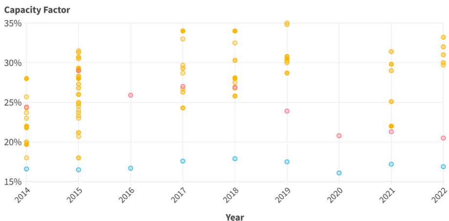
Fig. B.8. Capacity factors from solar PV projects in Brazil. Data sources: CCEE (2024); IRENA (2023).
